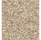
Gravel: Gravel is a budgetfriendly option that allows for excellent drainage, making it ideal for areas with heavy rainfall. While gravel driveways are easy to install, they require frequent maintenance to prevent ruts and keep the gravel in place.
