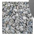
Crushed stone: Crushed stone driveways are similar to gravel but have a more uniform look. They offer excellent drainage and flexibility in design, though they can become uneven over time without regular upkeep.
